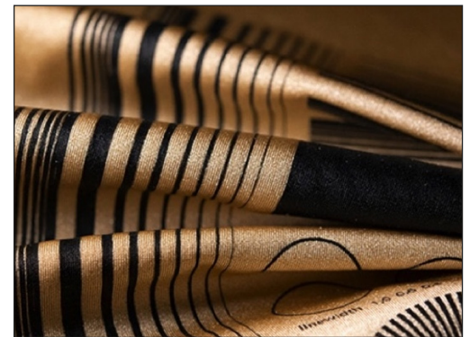
Stretchable sensors containing nanosilver and silicone allow greater flexibility and scalable production.
